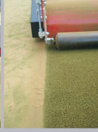
Removal of infill from a sand filled carpet
