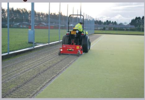
The **X-treme Clean** maintains synthetic turf systems that use sand as an infill mix for stability. The machine contains a set of firm brushes, which rotate in opposite directions. The infill is vigorously brushed, bringing it up to the turf surface.
