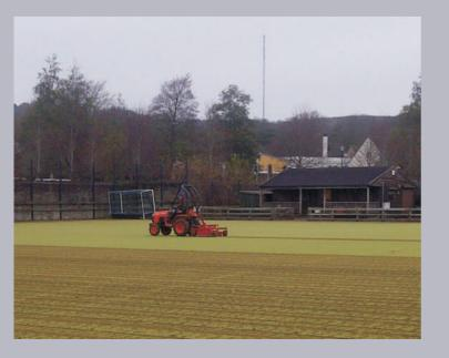
The brushes remove algae and moss, while de-compacting the top sand layer, making it more permeable and thus aiding surface drainage, and preventing separation of the infill mix.
