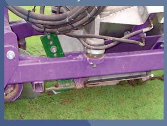
Pressure wheel on the machine pushes the cut edges together, thus closing the opening
